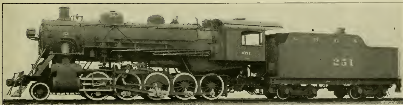
Decapod Type Locomotive for the Gulf, Mobile and Northern Railroad, Built by Baldwin Locomotive Works
